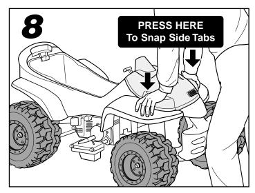
Press firmly on each side of the cowling to snap the four side tabs into the slots in the vehicle body. Make sure the rear tab stays aligned with the slots.
